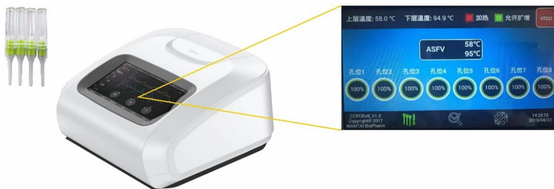
Fig. 1. Illustration of ASFV iiPCR device and PCR tube. The PCR tubes were put into the individual reaction chambers in the compact and portable iiPCR device. The reaction started when pushing the start button on the touch screen and the real-time process of reaction visualized in percentage appeared on the screen until the results shown with “+” for positive sample or “-” for negative sample. The iiPCR could be completed within 25 minutes.
